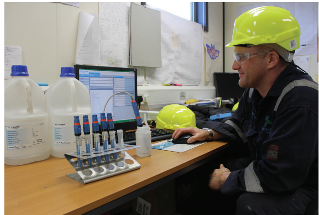
Sensors are calibrated away from the process under constant conditions.
